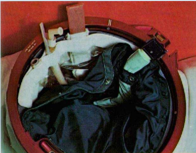
FIGURE 3.2 Neck ring of the Apollo space suit showing the In-suit food bar and the drink device (NASA photograph).
